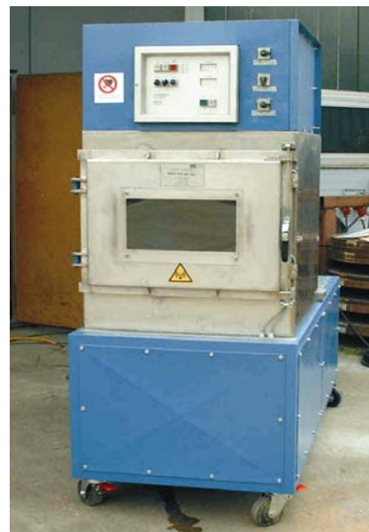
Microwave chamber with power of 6 kW, stepless controlable with exhaust air system.
