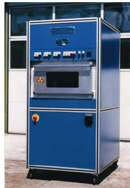
Microwave chamber drier with power of three times of 1,2 kW, switchable and stepless controlable.
