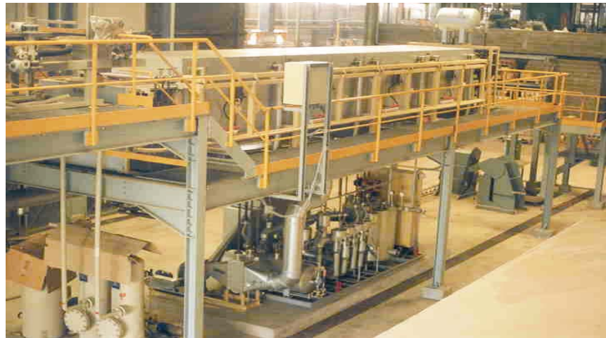
Contact belt drier above: thermal oil heated; below: electrical heated
