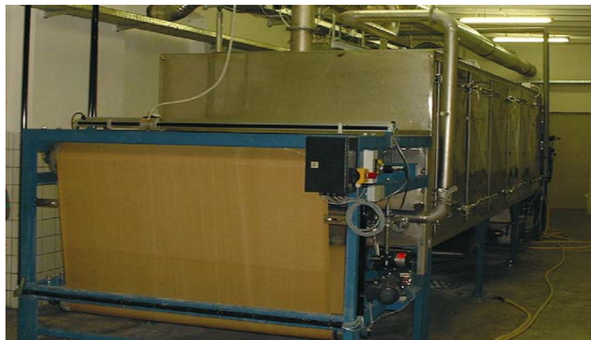
Contact belt drier above: thermal oil heated; below: electrical heated
