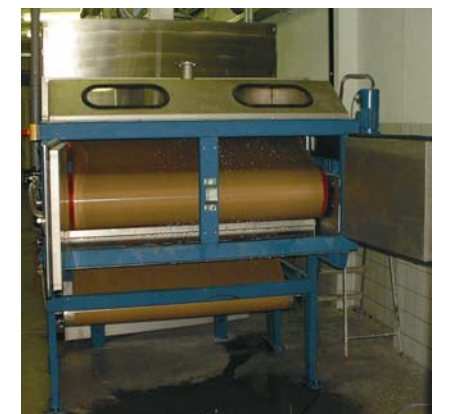
Discharge module with drive roller (above) and turning roller (below)
