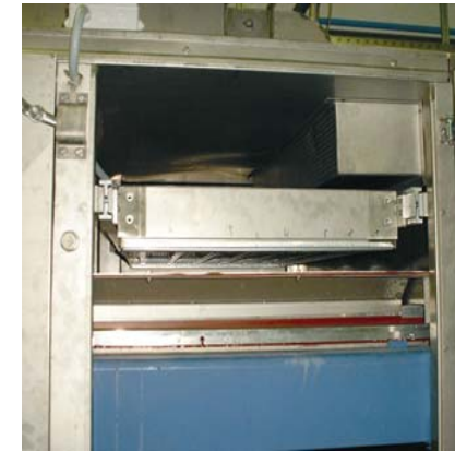
View inside drying chamber with additional infrared radiation heater
