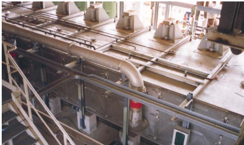
Convective belt drier in modular construction
