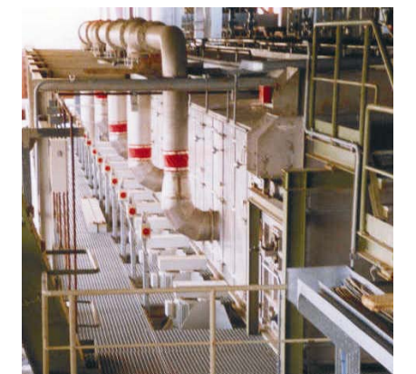
Two stage special belt drier with fresh air pipe and circulation air fan
