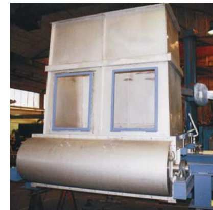
Bunker feeder with belt drive and maintenance doors
